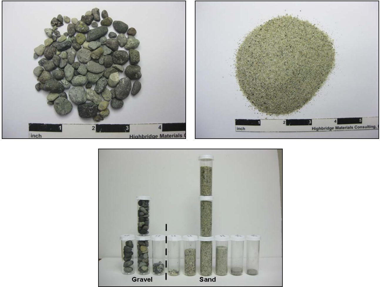
Figure 4: Photographs of the aggregate extracted through acid digestion. (Upper left) The gravel addition is shown. The volcanic particles are mostly rounded to subrounded in shape with aspects that range from equant to slightly oblate. (Upper right) The sand addition is shown. The sand is mostly uniform and light brownish gray in color. (Lower) The total aggregate is shown after gradation through a standard sieve stack. Note the distinctly bimodal distribution with a trough at around the No. 8 sieve that divides the gravel and the sand.
