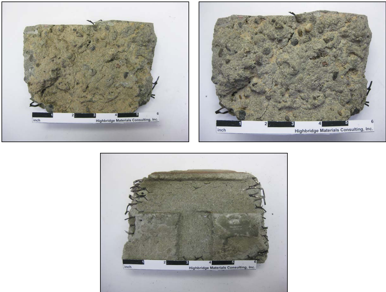
Figure 1: Photographs of the stucco sample received by Highbridge for examination. (Upper left) The outer face is shown as received. Note there is a soft, orange-toned coating covering most of the finish coat. (Upper right) The outer surface is shown after the laboratory scrubbed off the coating to reveal a weathered face with partially exposed aggregates. (Lower) The inner surface is shown. There are complete impressions of wood lath and another surface behind the lath.
