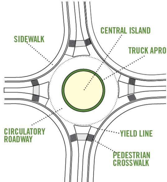
Roundabouts are designed to accommodate fire trucks and large vehicles.
